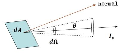
Mean Intensity  $J_{\nu} = \frac{1}{4\pi} \int I_{\nu} d\Omega$ Net Flux  $F_{\nu}$  [ergs s<sup>-1</sup> cm<sup>-2</sup> Hz<sup>-1</sup>]  $F_{\nu} = \int I_{\nu} \cos \theta \, d\Omega$ Total Flux  $F = \int F_{\nu} \, d\nu$
