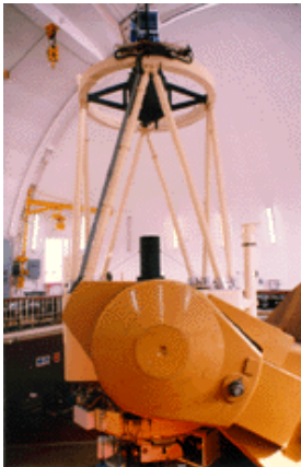
Isaac Newton Telescope at La Palma, Spain. D=2.5 m, with a polar-disk/folk type of equatorial mount
