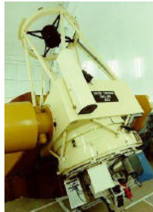
Isaac Newton Telescope at La Palma, Spain. D=2.5 m, with a polar-disk/folk type of equatorial mount
