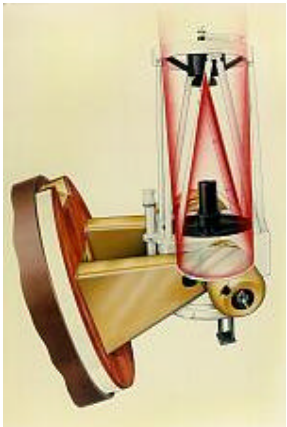
Isaac Newton Telescope at La Palma, Spain. D=2.5 m, with a polar-disk/folk type of equatorial mount
