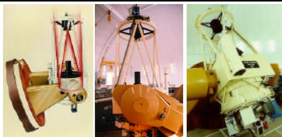
Isaac Newton Telescope at La Palma, Spain. D=2.5 m, with a polar-disk/folk type of equatorial mount
