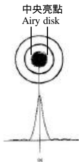
Diffraction pattern of a point source
