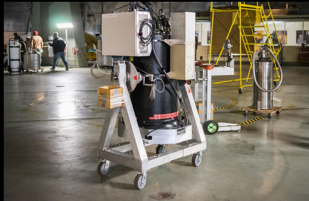
WIRC+Pol near-infrared spectropolarimeter at Palomar Observatory
