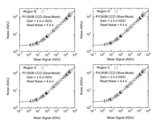
**Fig. 4** Signal and the noise of  $300 \times 300$  regions on the CCD for slow readout mode. Dotted curves are the fit using Eq. (3).
