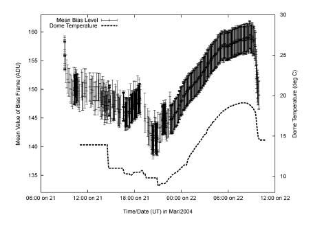
Fig. 2 Level of bias frame, plotted against data acquisition time in UT. The data are taken in the fast readout mode. The ambient temperature in the dome of the LOT is shown as the dotted line.
