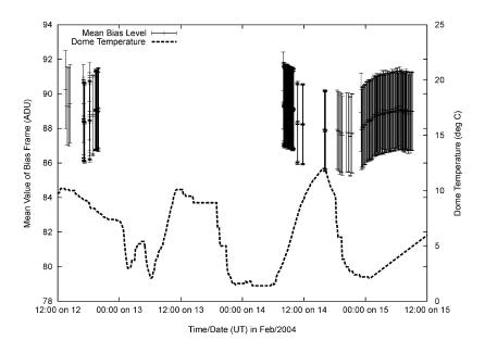
Fig. 1 Level of bias frame, plotted against data acquisition time in UT. The data are taken in the slow readout mode.
