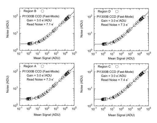
**Fig. 3** Signal and the noise of  $300 \times 300$  regions on the CCD for fast readout mode. The dotted curves are the fit using Eq. (3).
