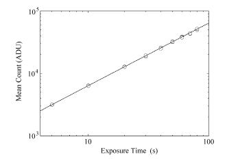
**Fig. 5** A plot of the exposure time versus mean count of the CCD. The light source is eight LEDs. The dotted line is the fit using Eq. (4).
